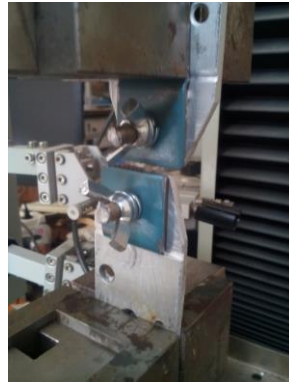
Specimen in the Zwick&Roell rupture machine
